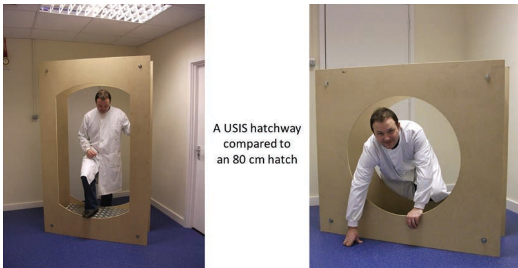
Fig. 3 USIS Passage Way (left) Compared with an 80 cm Passage Way (right).
